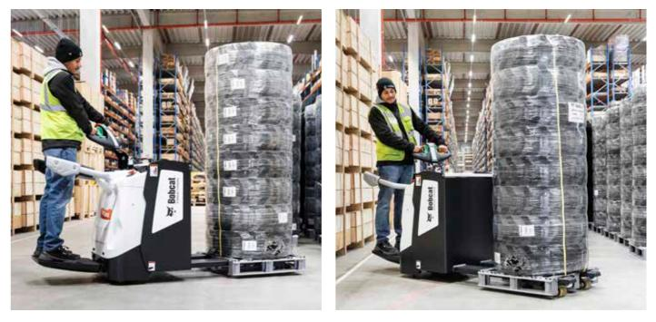
**TANDEM LOAD WHEELS AND EASY PALLET ENTRY** Contoured fork design and tandem load wheels allow easy entry into, and exit from, palletized loads.
