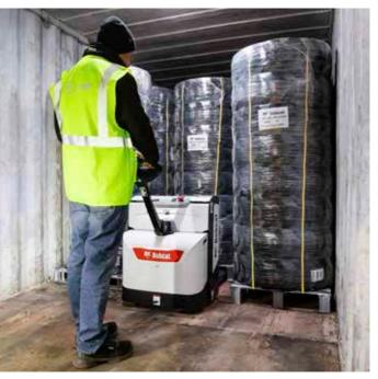
► SUB-ZERO STORAGE (-30 °C) Thanks to their specialized frame coating and hydraulic oil, these trucks continue running smoothly in temperatures as low as -30 °C, ensuring effortless and efficient work in cold conditions.
